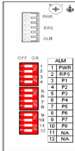
The plastic green colored contact power block (shown in the diagram to the left) is composed of six contacts and can be inserted and removed easily by hand to connect to the six pin terminal block receptor (male contacts located on the body of the Switch). The top two contacts (PWR) are designated for the primary DC input, while the middle two contacts (RPS) are for redundant DC input. The lower two contacts (ALM) are for connection to an external alarm.
