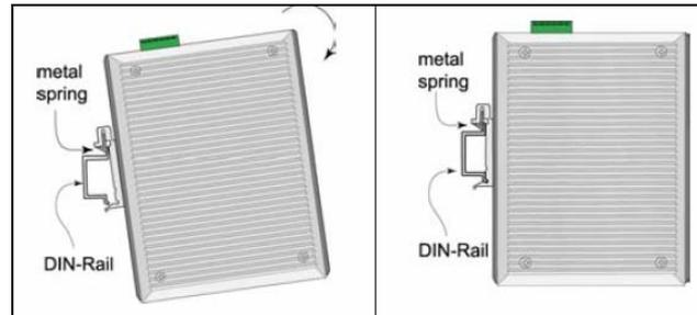
The setup of the Switch can be performed using the following steps:
